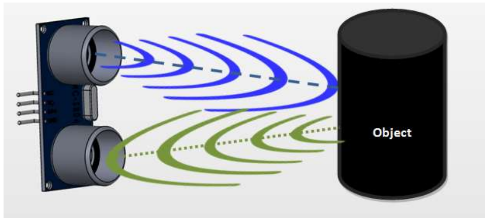
Fig 4.1: ultrasonic sensor working principle
